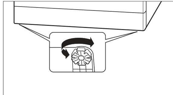
5. In order to equalise unevenness in the floor and set up the dishwasher on a level horizontal base, you can screw the four adjustable feet in or out. There are slots in the appliance feet around the circumference. Insert a screwdriver and turn the appliance foot. Use a spirit level to set up the dishwasher.
