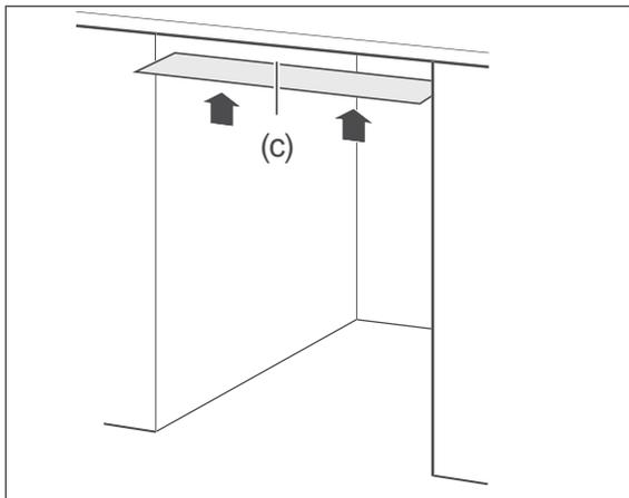
3. Affix the enclosed condensation-protective film (c) to the bottom of the work surface. In this way, you will avoid damage to the work surface caused by hot steam emitting from the dishwasher when the door is opened.
