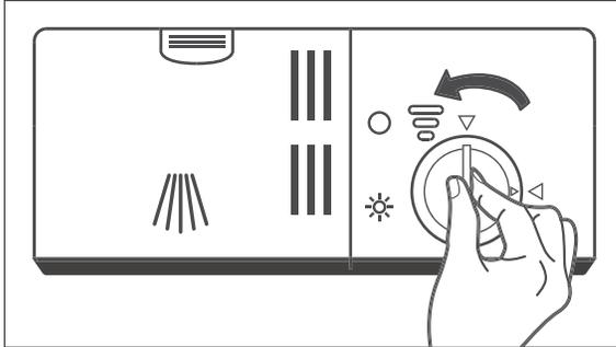
1. Turn the catch of the rinse aid dispenser (20) a quarter turn in an anticlockwise direction and remove it.
