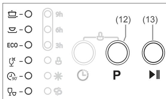
You can interrupt an active dishwashing programme at any point and start a new one. However, do not forget to add extra dishwasher detergent if the programme has already been running for a longer period and the cover of the dishwasher detergent compartment is already open.
