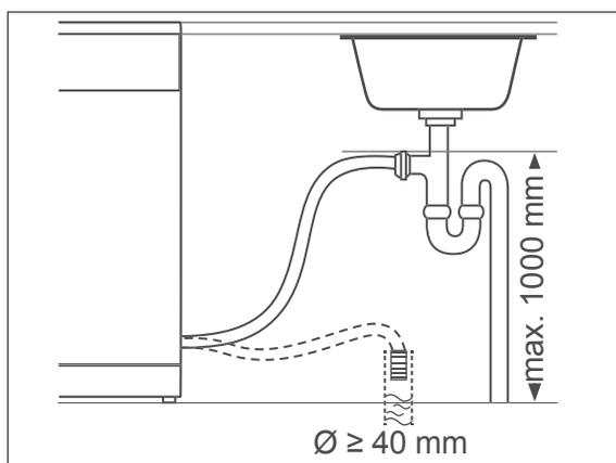
The outlet hose (22) can be connected in two ways:
