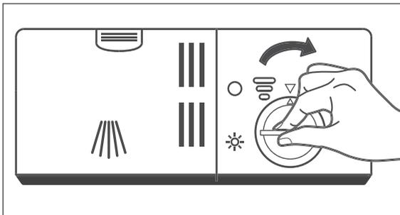
4. Insert the rinse aid dispenser catch (20) and give it a quarter turn clockwise. The markings on the lid and the rinse aid dispenser (20) must be aligned upon insertion.
