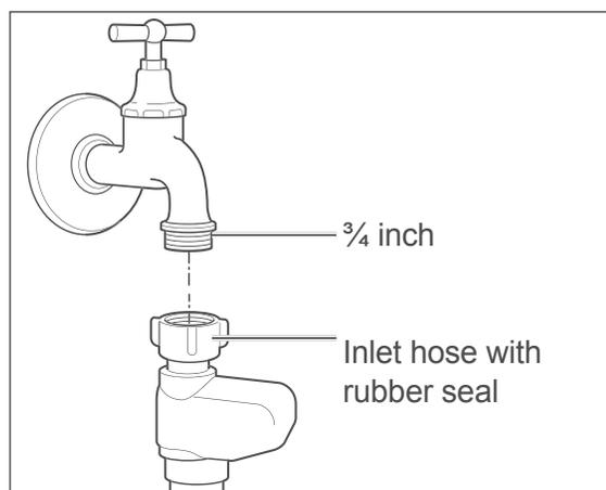
For water supply, you need a water tap with a  $\frac{3}{4}$  inch screw connector.
