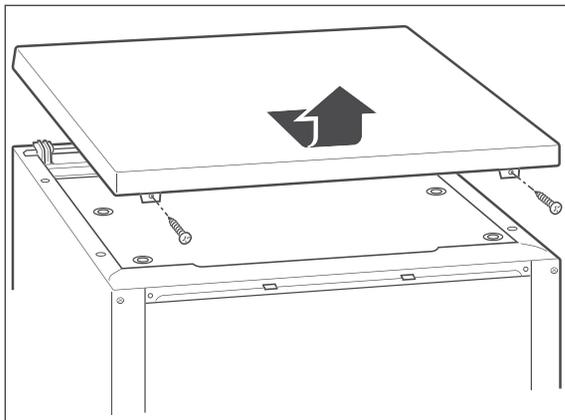
2. Loosen both screws on the reverse side of the covering panel and remove them.
