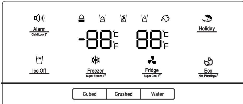
When the appliance is powered on for the first time, the backlighting of the icons on the display panel starts working. If no buttons have been touched and the doors are closed, the backlighting will turn off after 60 seconds.
