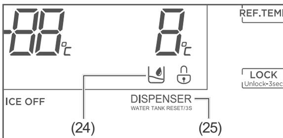
1. To dispense cold water, press the DISPENSER button (25) repeatedly until the
