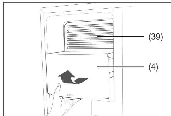
3. Lift the ice cube container slightly (4) and pull it out, keeping it level.
