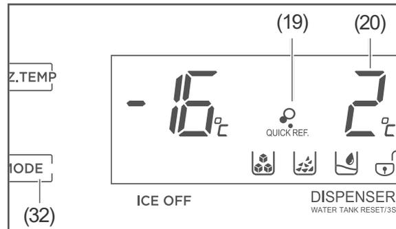
Select the 'Quick refrigerating' mode QUICK REF (19) when you want to cool a can more quickly in the refrigerator, for example.
