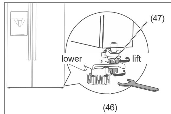
2. Turn the locknut (46) two full rotations clockwise to loosen it. Use the spanner supplied to do this.
