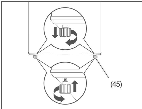
2. Level out any unevenness on the ground using the two front screw feet (45).
