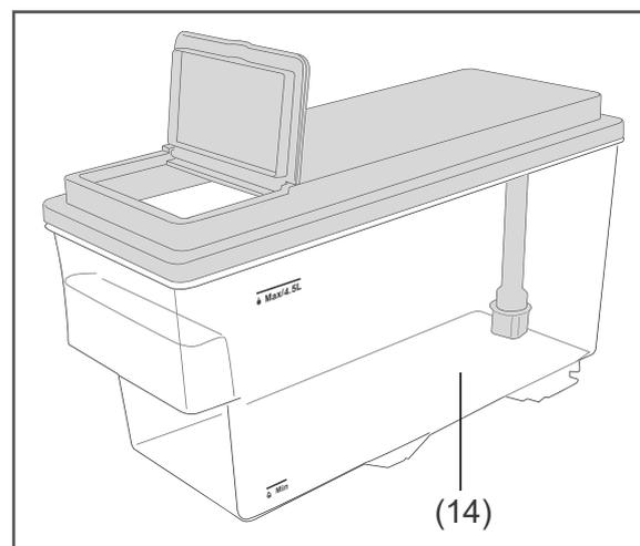
1. Open the lid and fill the water tank (14) with cold, fresh tap water so that the water level is above the 'Min' mark but below the 'Max' mark (4.5 L).
