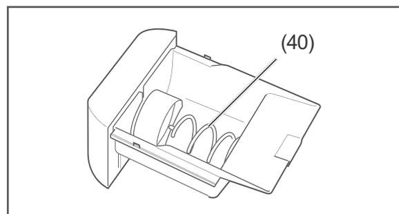
1. Dispose of any ice cubes down the drain. If necessary, turn the conveyor screw (40) clockwise or anticlockwise to loosen any trapped ice cubes.
