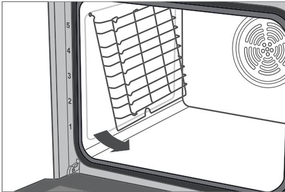
2. Pull the bottom of the oven rack guide approx. 45° away from the wall so that you can remove it.
