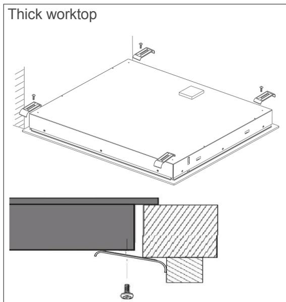
5. Depending on the worktop's thickness, attach the 4 brackets by screwing them to the hob from below. This will prevent the hob from moving.
