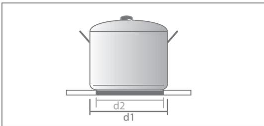
The **d1** diameter is always provided as a pan and pot size. **d2** base diameter is always around 2 cm smaller. Pots that are too big can cause paintwork damage.
