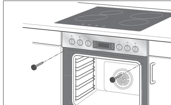
5. Screw the oven to the built-in cabinet with the two screws which have been supplied.
