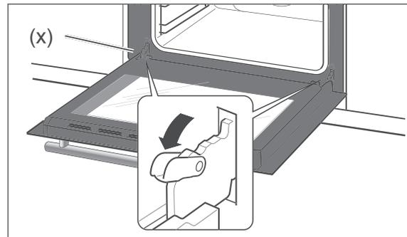
2. Fold the clips (x) on both sides all the way forward. Use a screwdriver if necessary.
