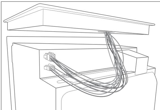
2. Insert the hob plugs into the sockets on the top of the cooker. Do not use any force. The plugs are coded. Polarity reversal is therefore not possible.
