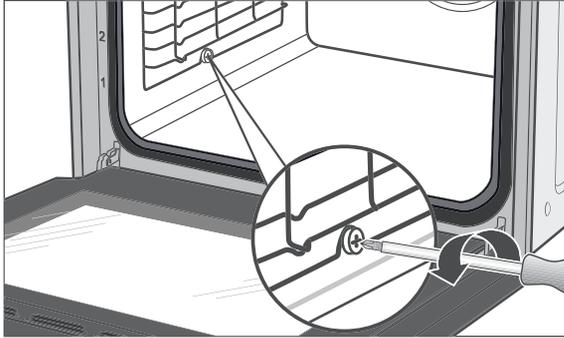
1. Loosen the screws of the baking tray guides and remove them.
