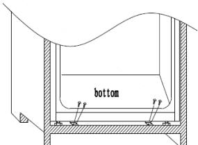
Fit the seal to the appliance, cut off the excessive part if necessary. Fit the bottom parts with plastic covers.
