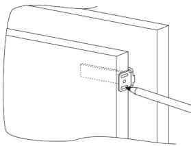
Connect the appliance door to the cabinet panel keeping the loader slots as guidelines.
