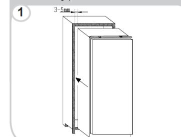
After ensuring the match between appliance door and column door, then screw the appliance upper part to the cabinet
