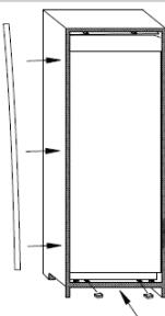
Mark the fixing points for the screws and drill with a bit of a diameter of 2.5mm.
