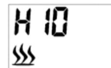
Press button E or F to set the hour of the activation time. Press button C to validate.
