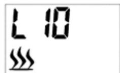
If the set temperature is higher than the room temperature detected by appliance, the heating starts. The heating will not start if the set temperature is lower than the room temperature.
