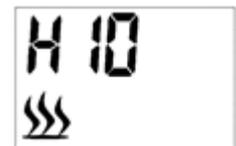
Press button E or F to adjust temperature. If the set temperature is higher than the room temperature detected by appliance, the heating starts. The heating will not start if the set temperature is lower than the room temperature.
