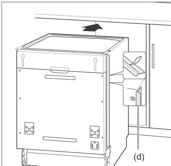
5. Remove the protective films from the side end profiles (d).
