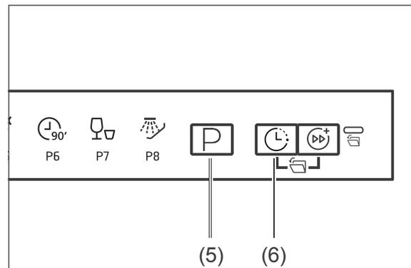
2. Press the **P** button (5) for 5 seconds within 60 seconds of switching on.
