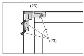
9. Screw the supplied upper hinge for the left stop (26) using the screws (23).
