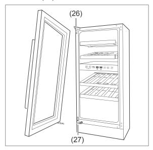
11. Place the glass door first in the top hinge (26), then in the bottom hinge (27). Close the glass door.
