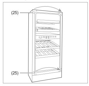
8. Remove the 6 dummy plugs (25) from the threaded holes above and below and place them into the threaded holes on the opposite side.
