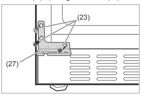
10. Screw the supplied lower hinge for the left stop (27) on the other side using the screws (23).
