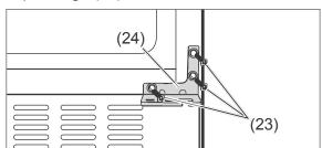
7. Unscrew the three screws (23) on the lower hinge (24) and remove it.
