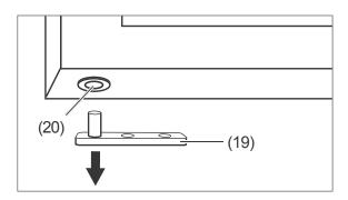
4. Pull the hinge plate (19) out of the plastic insert (20) at the bottom edge of the glass door.
