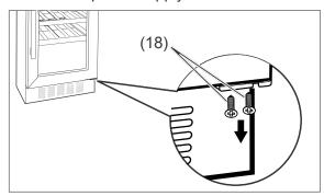
2. Unscrew the two screws (18) from the lower hinge.
