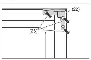
6. Unscrew the three screws (23) on the upper hinge (22) and remove it.
