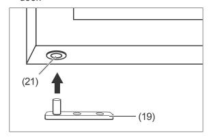
5. Rotate the glass door 180° and place the hinge plate (21) into the plastic insert (19) here.
