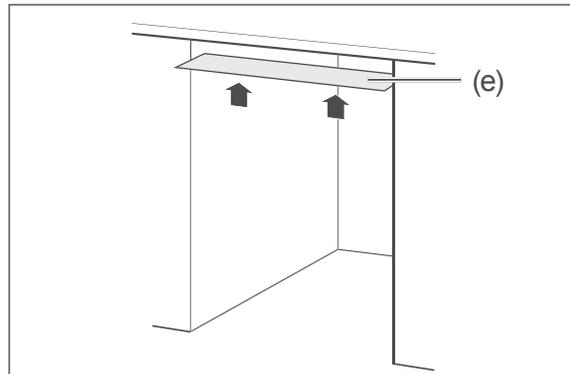
4. To protect the worktop against condensation, affix the enclosed protective film (e) to the underside of the worktop. This will help you minimise damage to the worktop from the outflow of hot steam.
