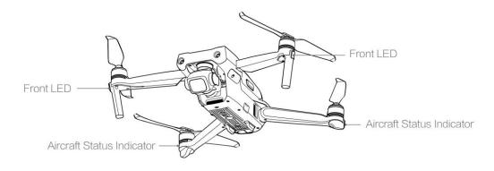
The front LEDs show the orientation of the aircraft and glow solid red when the aircraft is turned on to indicate the front of the aircraft.
