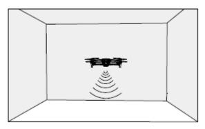
If the aircraft is in Normal or Cine mode and Obstacle Detection is enabled in DJI Fly, the Forward, Backward and Upward Vision Systems will activate automatically when the aircraft is powered on. Using the Forward, Backward and Upward Vision Systems, the aircraft can actively brake when detecting obstacles. The Forward, Backward and Upward Vision Systems work best with adequate lighting and clearly marked or textured obstacles.
