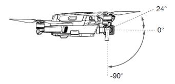
Use the gimbal dial on the remote controller to control the tilt of the camera. Alternatively, enter the camera view in DJI Fly. Press the screen until an adjustment bar appears and drag up and down to control the camera's tilt.
