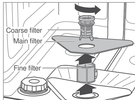
Check the coarse filter, the main filter and the fine filter after each rinse cycle and remove food residues and foreign bodies if necessary:
