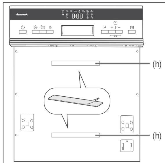
9. With the protective film removed, affix the hook-and-loop strips to the middle of the recessed areas on the dishwasher door.
