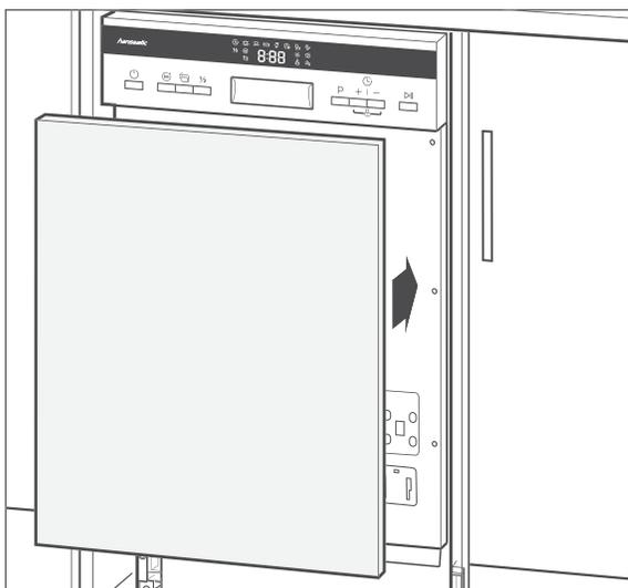
16. Fix the front panel to the dishwasher door using the hook-and-loop strips (i), hold it firmly and carefully open the door.
