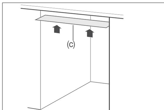
3. Affix the enclosed condensation-protective film (c) to the bottom of the work surface. In this way, you will avoid damage to the work surface as a result of hot steam which may be emitted from the dishwasher if the dishwasher door is left open.
