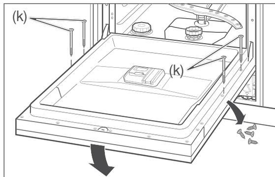
17. Remove the 4 screws from the inside of the door. Screw the front panel in place at these positions using the 4 enclosed screws (j).
