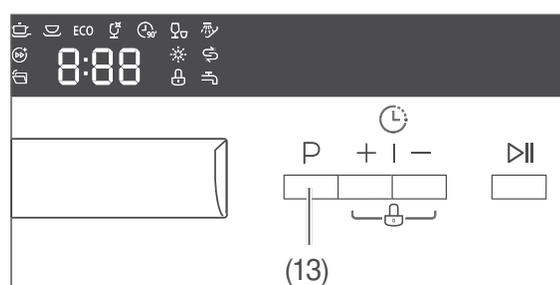
2. Press and hold the **P** button (13) for as long as required until the current water hardness is shown on the display: H 1 to H 6.
