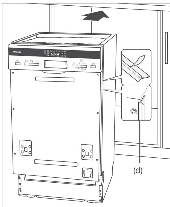
5. Remove the protective films from the side end profiles (d).
