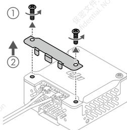
2. Use an appropriate tool (tweezers) to disconnect and lift the plugs, and then remove the antenna.
