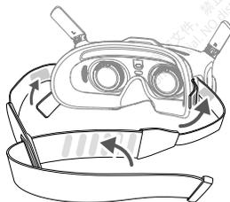
4. After the devices are powered on and the image transmission is displayed, wear the goggles and adjust the headband until the goggles fit comfortably.
