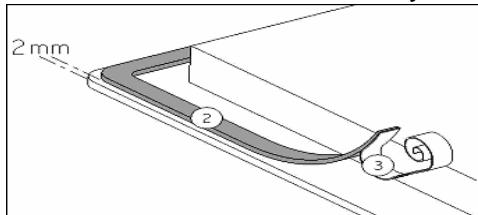
Stick the gasket (2) two millimeters from the external edge of the glass, after removing the protection sheet
