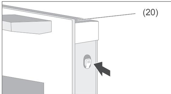
2. To remove the cover (20), push the bolts in lightly on both sides.
