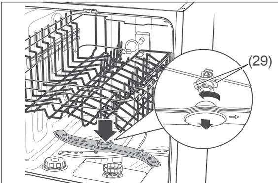
3. The upper spraying arm is affixed using a bayonet closure. To remove the spraying arm, hold the two serrated bayonet grips (29) still and turn the spraying arm clockwise.
