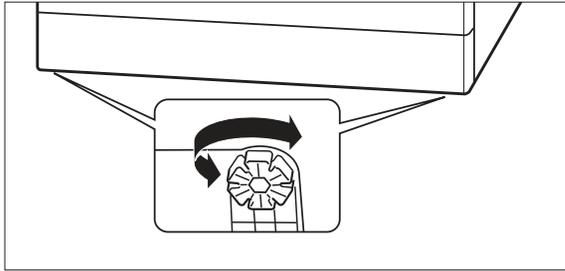
5. In order to equalise unevenness in the floor and set up the dishwasher on a level horizontal base, you can screw the four adjustable feet in or out. There are slots in the appliance feet around the circumference. Insert a screwdriver and turn the appliance foot.
