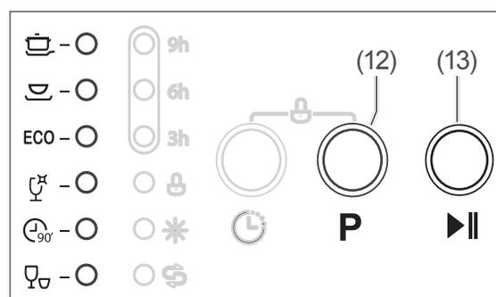
2. Press the **P** button (12) repeatedly until the LED to the right of the desired programme symbol lights up.
