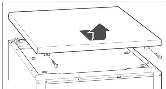
2. Loosen both screws on the reverse side of the covering panel and remove them.
