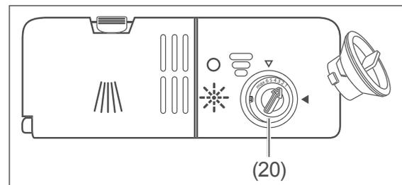
1. Turn the cover of the dishwasher salt compartment (20) a quarter turn in an anti-clockwise direction and remove it.
