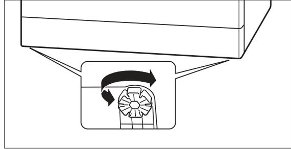
3. In order to equalise unevenness in the floor and set up the dishwasher on a level horizontal base, you can screw the four adjustable feet in or out. There are slots in the appliance feet around the circumference. Insert a screwdriver and turn the appliance foot.
