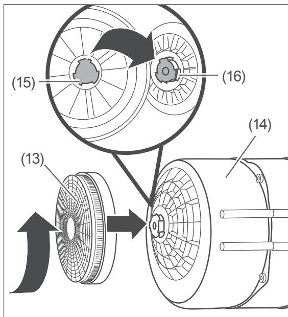
4. Only when replacing the charcoal filters: The two activated charcoal filters (13) are located to the right and left of the motor (14). Loosen the two activated charcoal filters (13) and remove them.
