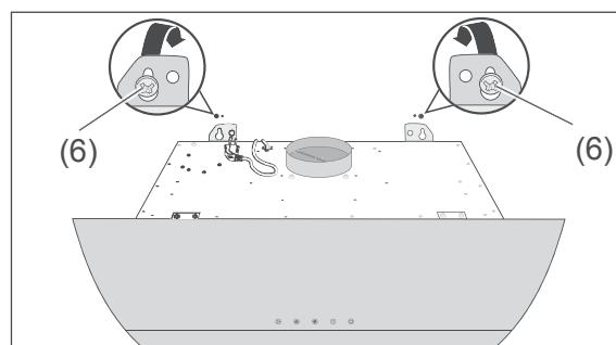
3. Carefully mount the exhaust hood on the two round-head screws (6) on the keyhole openings.
