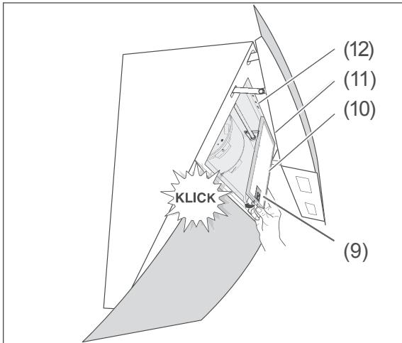
5. Place the grease filter (10) with the pins (11) into the openings (12).
