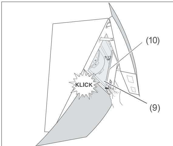
6. Place the grease filter (10) with the pins into the openings.
