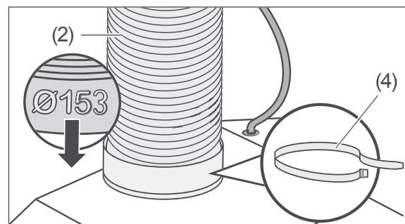
1. Insert the end of the exhaust air hose (2) with the larger diameter (153 mm) into the connection with the check valve (3).
