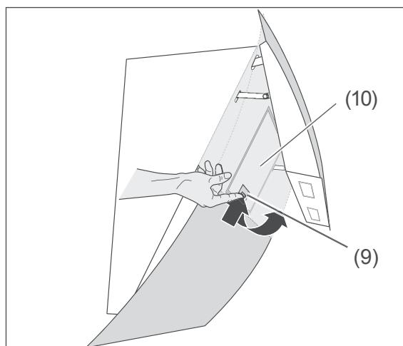
3. Open the locks (9) on the grease filter (10) and carefully remove the grease filter (10).
