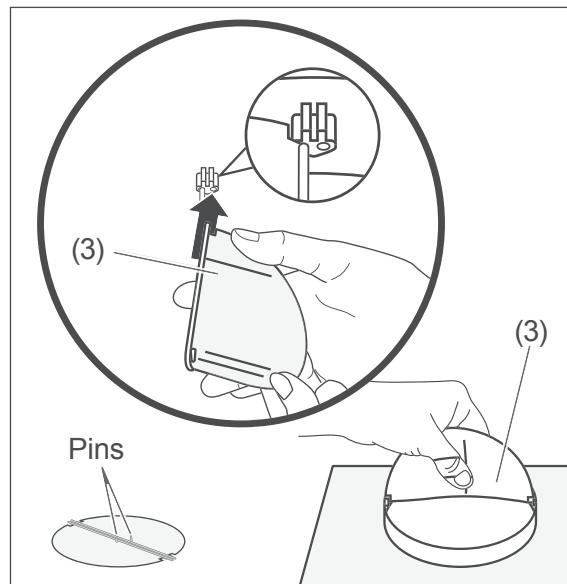
1. Place the two halves of the check valve (3) into the opening on the top of the exhaust hood (1).
