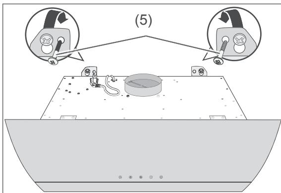
5. Turn two round-head screws (5) into the prepared wall plugs to secure the exhaust hood and screw the exhaust hood tightly to the wall.
