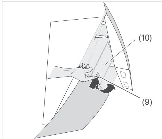
3. Open the locks (9) on the grease filter (10) and carefully remove the grease filter.
