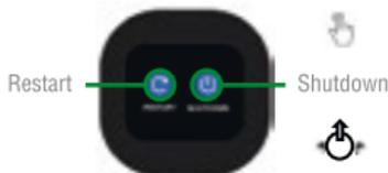
**Long press for 10 seconds:** Restart the system (display the startup screen).
