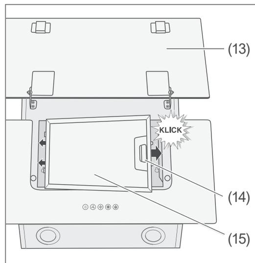
8. Place the grease filter (15) with the pins into the openings.
