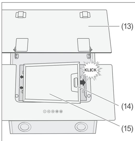
7. Place the grease filter (15) with the pins into the openings.
