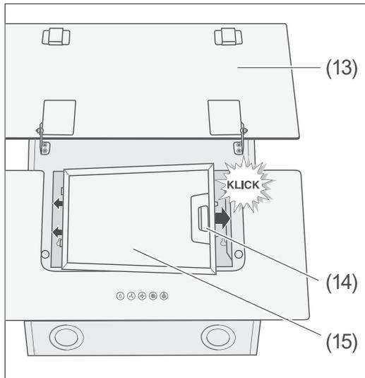
5. Place the grease filter (15) with the pins into the openings.
