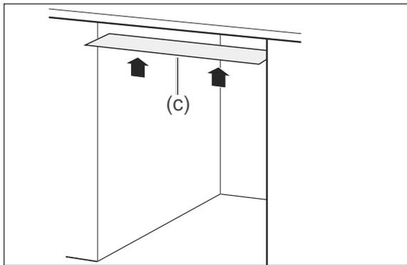
3. Affix the enclosed condensation-protective film (c) to the bottom of the work surface. In this way, you will avoid damage to the work surface as a result of hot steam which may be emitted from the dishwasher if the dishwasher door is left open.
