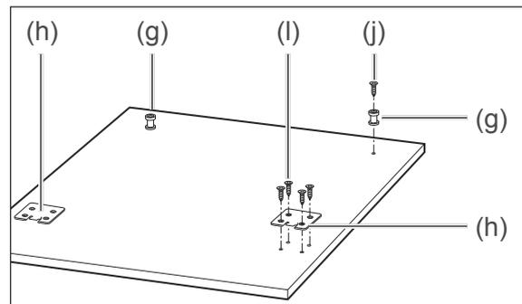
4. Affix both installation hooks (h) with four screws (l) each onto the front panel.
