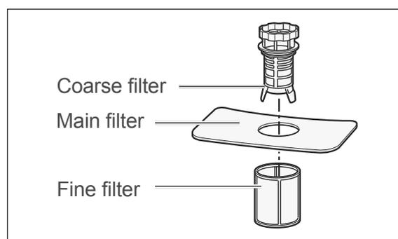
Check the coarse filter, the main filter and the fine filter after each rinse cycle and remove food residues and foreign bodies if necessary:
