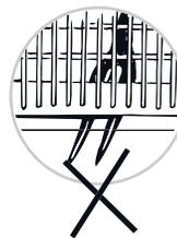
When loading the cutlery, ensure that it does not protrude through the bottom of the cutlery basket. Otherwise, the lower spraying arm will be blocked.
