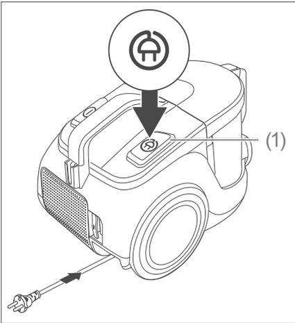
3. To retract the mains cord (11), press your foot down on the foot switch for the cable retractor (1). To avoid a 'whipping effect', hold the mains plug on the mains cord in your hand.
