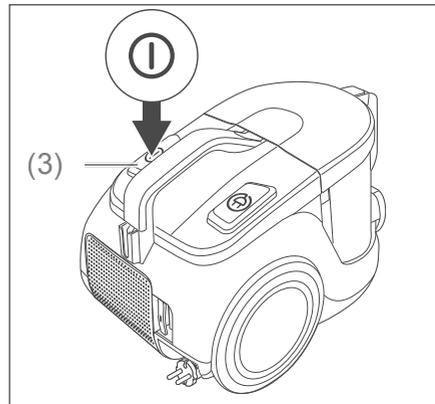
1. Use your foot to press the on/off foot switch (3) to switch the appliance off.
