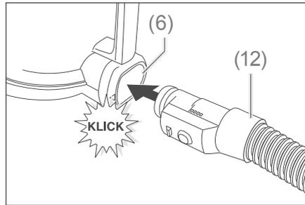
2. Put the suction hose (12) with the connector in the opening for the suction hose connection (6).
