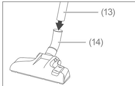
3. Select the desired nozzle (e.g. the floor nozzle) (14) and insert it into the telescopic tube (13).
