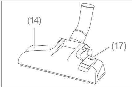
You will work with the floor nozzle (14) most of the time as it is designed for large, flat surfaces.
