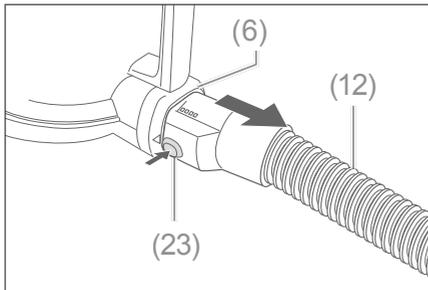
2. Pull the suction hose (12) out of the opening of the suction hose connection (6). First press the locking mechanism (23) and then remove the suction hose.
