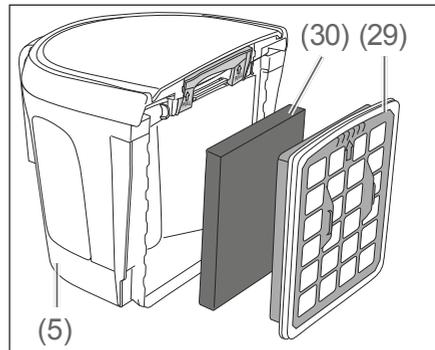
3. Remove the foam filter frame (29) and the foam filter (30).
