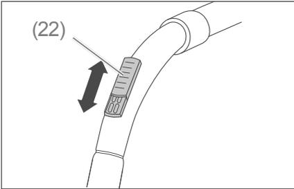
You can adjust the suction force as needed by using the air by-pass vent (22). The covering of the air by-pass vent (22) can be adjusted as desired.
