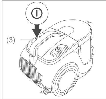
3. Use your foot to press the on/off foot switch (3) to switch the appliance on.
