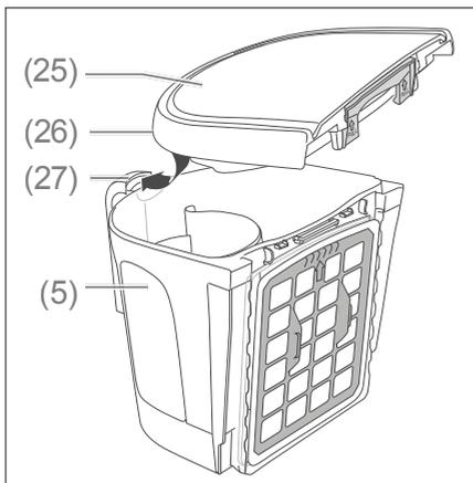
6. Place the dust bin lid (25) back onto the dust bin. Make sure that the mounting bracket (26) on the dust bin lid clicks into the opening (27) on the dust bin handle.
