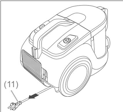
1. Pull the mains cord out by the mains plug (11) until the yellow marking is visible on the mains cord.
