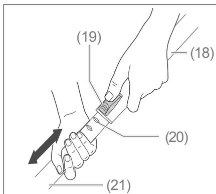
4. The length of the telescopic tube (13) can be adjusted to suit the height of its user.
