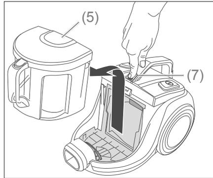
3. Press the unlocking button for the dust bin (7) and remove the dust bin (5) using the handle.
