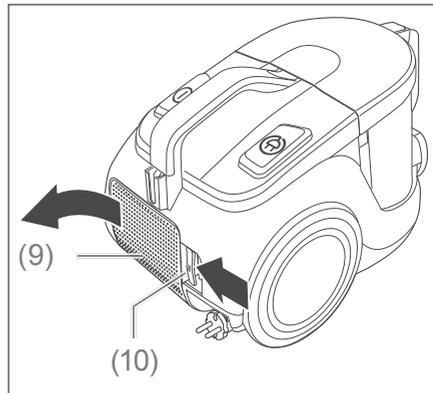
2. Remove the filter cover (9). To do this, press the the release mechanism (10)
