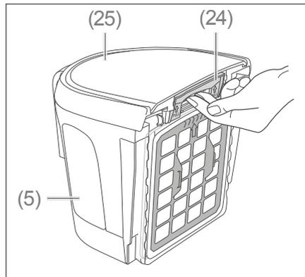
4. Release the locking mechanism (24) under the dust bin lid (25) and remove the dust bin lid (5).
