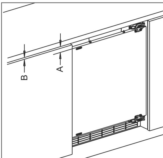
The brackets must be positioned 130 mm from the centre of the cabinet front panel.
