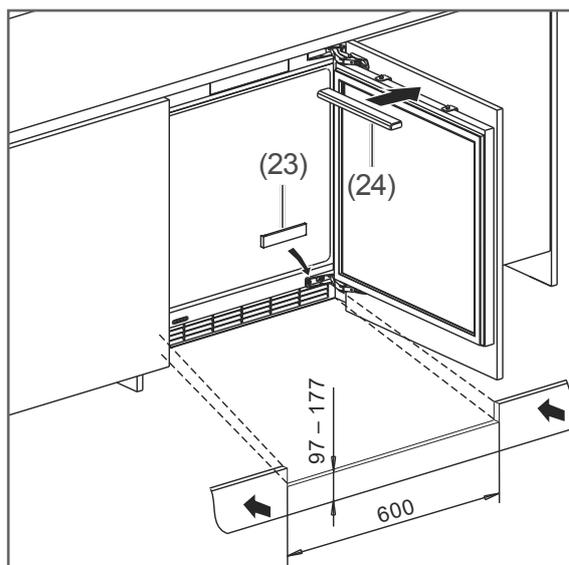
19. Put the screw cover (24) over the double-ended screws.
