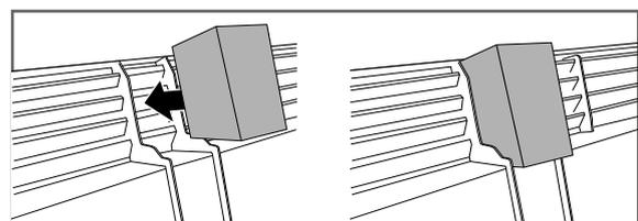
5. Remove the front panel (6) and insert the separation foam (20) in the middle of the front panel.
