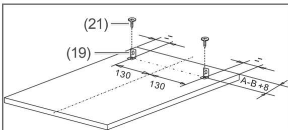
10. Fasten the brackets (19) to the cabinet front panel using the screws (21).
