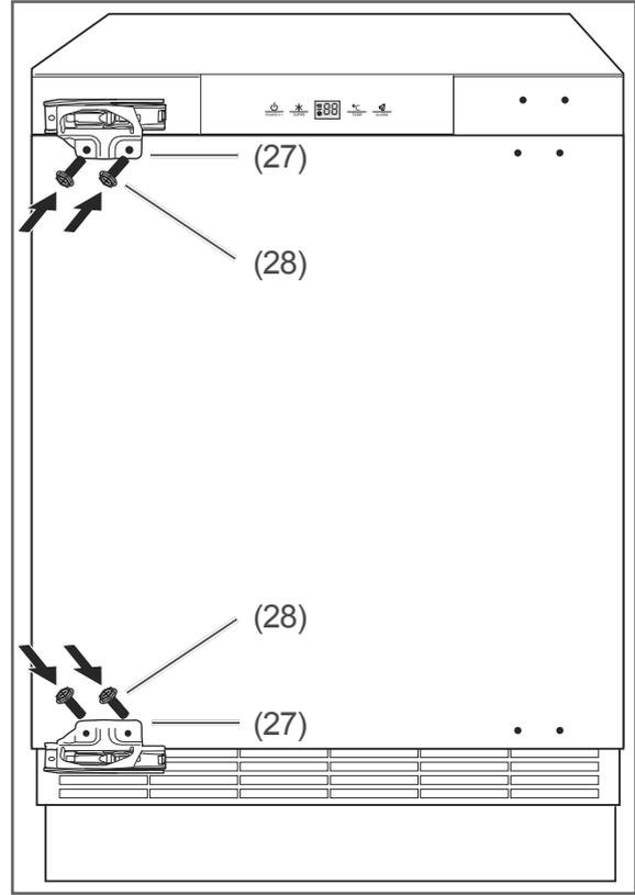
6. Fasten the hinges (27) using the screws (28).
