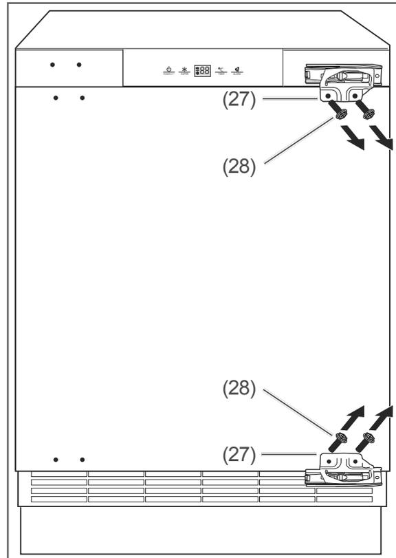
3. Loosen the screws (28) on the hinges (27).
