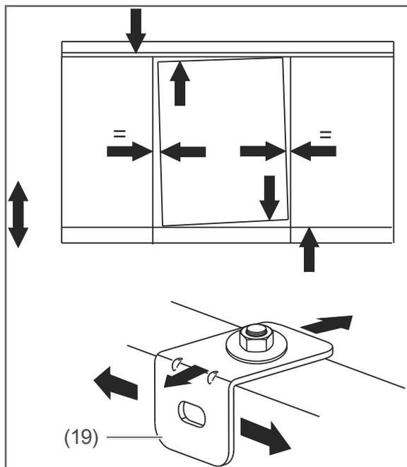
14. Align the bracket (19) such that the cabinet front panel is level.
