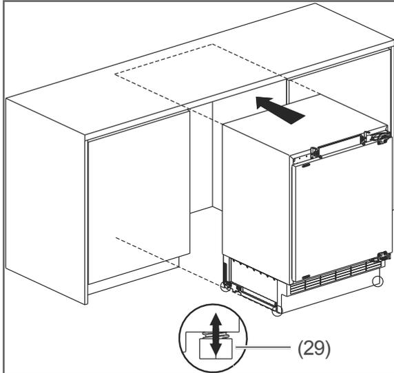
7. Level the appliance by adjusting its screw feet (29) to the right height.
