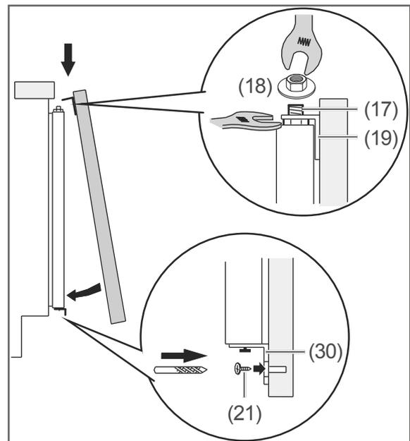
11. Attach the cabinet front panel to the double-ended screws (17) using the brackets (19).
