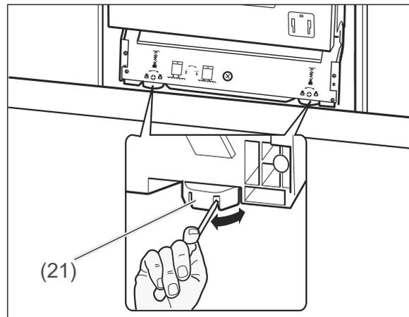
8. To position the dishwasher so that it is level, the two front adjustable feet (21) and the back foot on the appliance can be adjusted by up to 50 mm.
