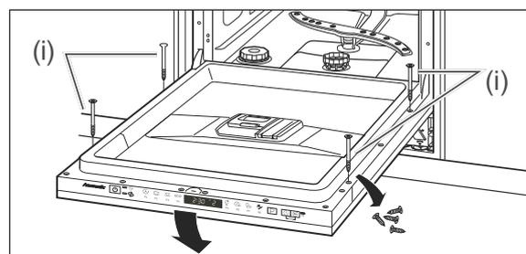
7. Remove the 4 screws from the inside of the door. Screw the front panel in place at these positions using the 4 enclosed screws (i).
