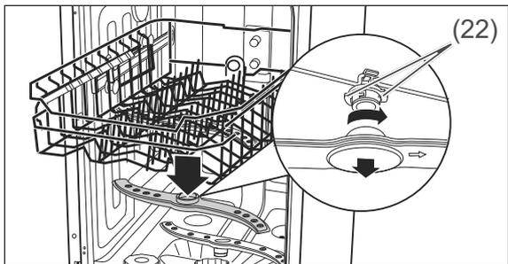
3. The upper spraying arm is affixed using a bayonet closure. To remove the spraying arm, hold the two serrated bayonet grips (22) still and turn the spraying arm clockwise.
