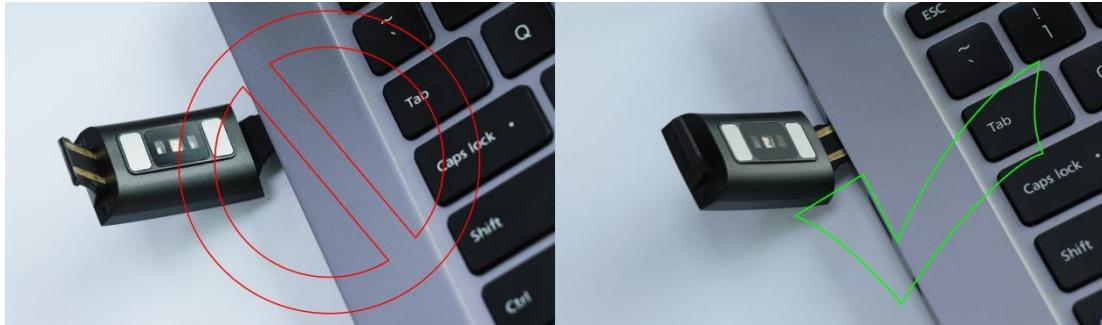
**Important:** Of the two ends of the watch strap, only one is the USB connection. Do not use the other end as it may damage the watch.
