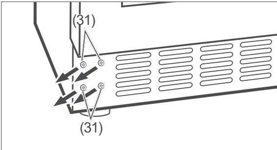
1. Loosen the screws (31) on the lower left of the appliance frame.
