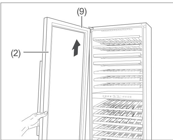
2. Rotate the glass door (2) until the hinge plate is on the lower side of the glass door and insert it into the upper hinge (9) for the left hinge side.
