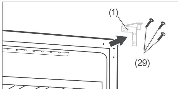
6. Loosen the screws (29) on the upper hinge for the right hinge side and remove the hinge.
