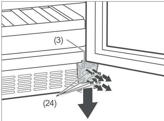
3. Loosen the screws (24) on the lower hinge (3) and remove the lower hinge (3). **Make sure to have at least one other person hold the glass door!**
