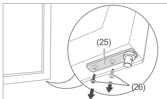
1. Loosen the screws (26) from the hinge plate (25) on the underside of the glass door's frame.
