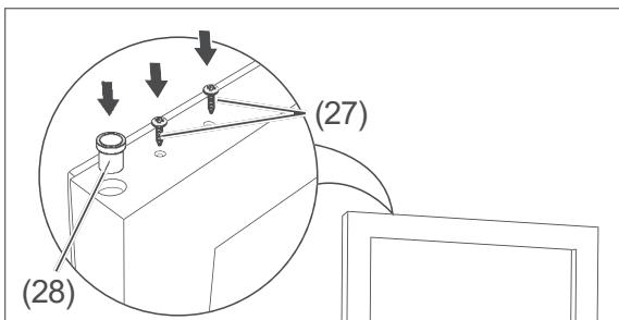
5. Loosen the screws (27) on the opposite narrow side of the glass door's frame, and insert the sleeve (28) into the holder on that side.
