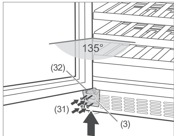
4. Put the lower hinge (3) against the appliance housing, making sure the axis (32) of the hinge plate (25) aligns with lower hinge's left hole (3). Then screw down the lower hinge (3) using the screws (31).
