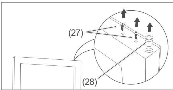
3. Loosen the screws (27) on the opposite narrow side of the glass door's frame, and remove the sleeve (28).
