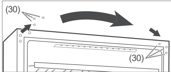
7. Remove the blind plugs (30) and insert them into the screw holes on the opposite side.
