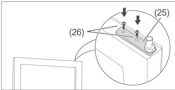
4. Place the hinge plate (25) on the opposite side of the glass door and secure it using the screws (26).
