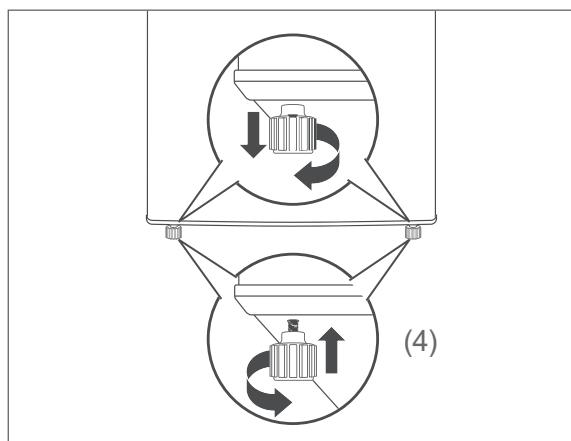
3. Level out any unevenness on the ground using the four screw feet.
