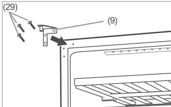
8. Screw the upper hinge (9) for the left hinge side onto the appliance using the screws (29).
