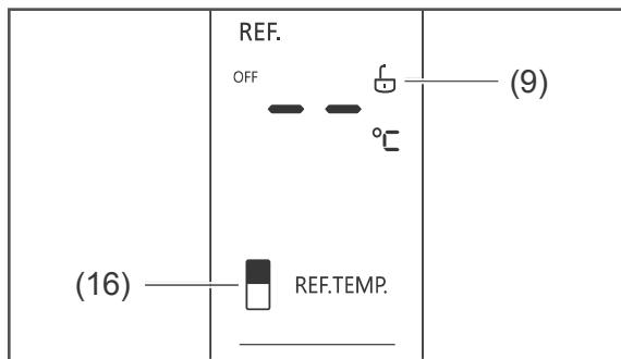
2. Switch the fridge off by pressing the sensor button REF.TEMP. (16) until two dashes and 'OFF' appear in the display. A short time later, the temperature of the freezer and '--' will be displayed alternately. As a result the fridge is switched off.
