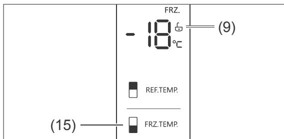
2. Tap the sensor button FRZ.TEMP. (15) repeatedly to set the desired temperature. Possible settings: -24 °C to -16 °C.
