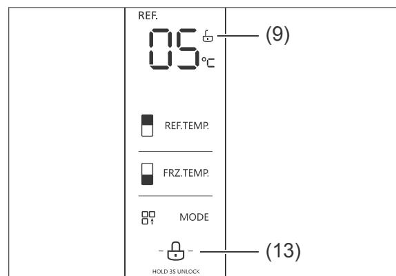
To change the settings, you first have to unlock the sensor buttons. To do this press the sensor button UNLOCK (13) until the indicator
