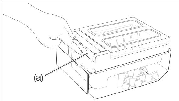
3. To remove the ice cubes, press the button (a) down firmly.
