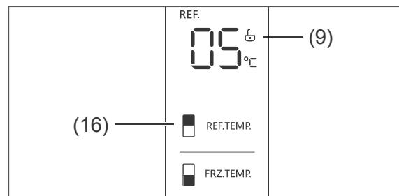
2. Tap the sensor button REF.TEMP. (16) repeatedly to set the desired temperature. Possible settings: +2 °C to +8 °C.
